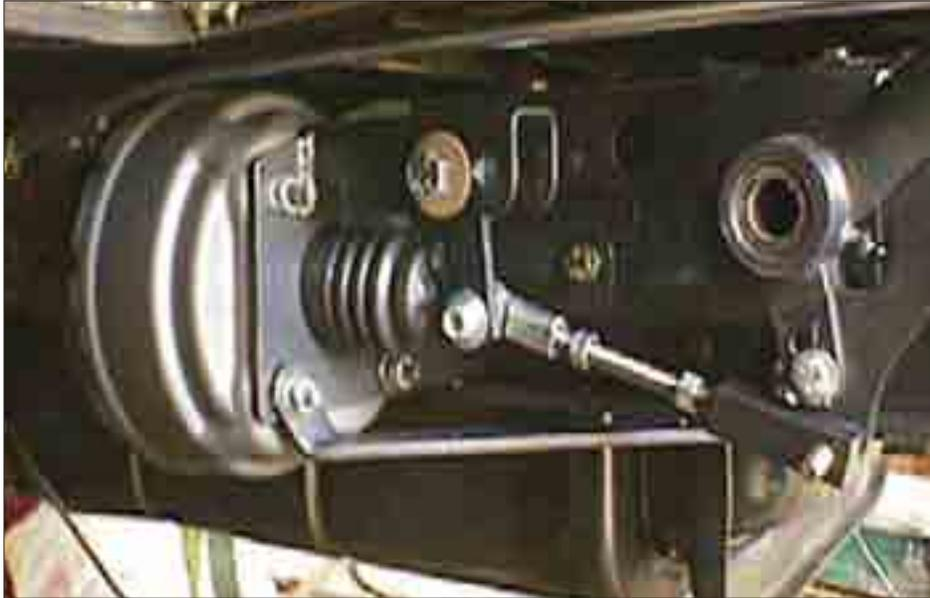
Power-brake mechanism of an automobile
