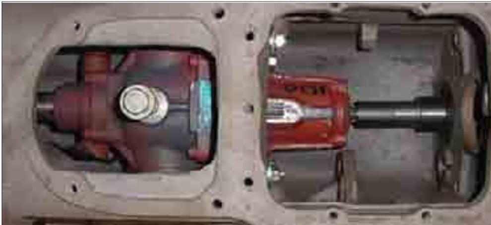
Hydrostatic transmission inside a tractor engine
